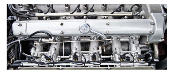
Having already completed many track days in his DB5, our client came to Aston Workshop looking for extra speed and refinement. The car was producing good power and torque with its triple 50 DCOE Webers and uprated 4.7 litre engine.
